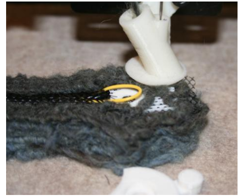
Figure 8. Partially printed arm example showing embedded components. Here we can see an embedded black nylon mesh tube (left) which holds a yellow tendon wire. This wire loops around a bolt which attaches the (white) assembly under it that is being printed over at this point. This assembly contains an embedded metal nut, nylon mesh to spread forces from the hard attachment point and 3D printed stiffening material.
